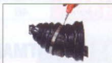
6. Install stainless clamp out of CV boot after adjust drive shaft to proper position. Last, cut rest CV boot along the tangent.
